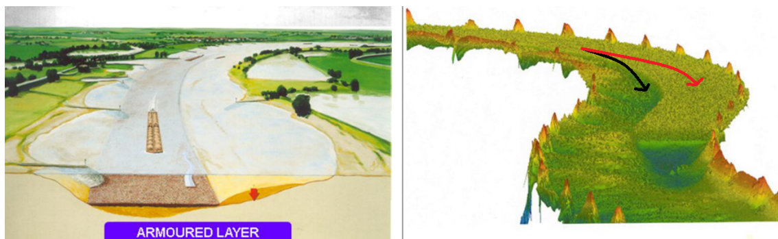
Figure A.3: Fixed layer, red arrow: water flow before construction of fixed layer, black arrow: water flow after construction of fixed layer (Havinga, 2016)
