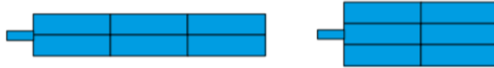
Figure J.3: CEMT-class VIc type of convoy; Left: 2x3; Right: 3x2. (Koedijk et al., 2017)
