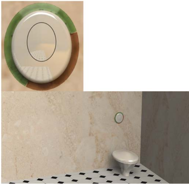
Figure E12. Smart lavatory system that supports the creation of awareness concerning energy and water usage.
