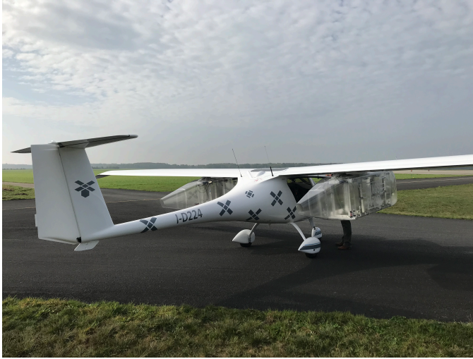
Figure 3.22: The aircraft used for detection, with the cargo boxes under the wings
