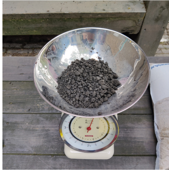
Step 1 / Choose your mix ratio. To start I used 70% sand 20% dredging specie and 10% cement, recommended by expert. Later I experiment with replacing sand with dredgingspecie and cement.
