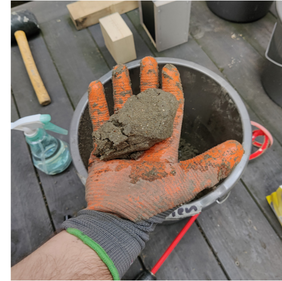
Step 3 / The water content has a direct impact on the strength of the finished wall. Too little water causes the wall to not be as compacted and become brittle. Too much water and the mix will be too wet and the water itself resists compaction. The mix should have a moist, rained upon consistency. This is easiest achieved by spraying the water in a fine mist instead of pouring it as you would in a normal concrete wall mix.
