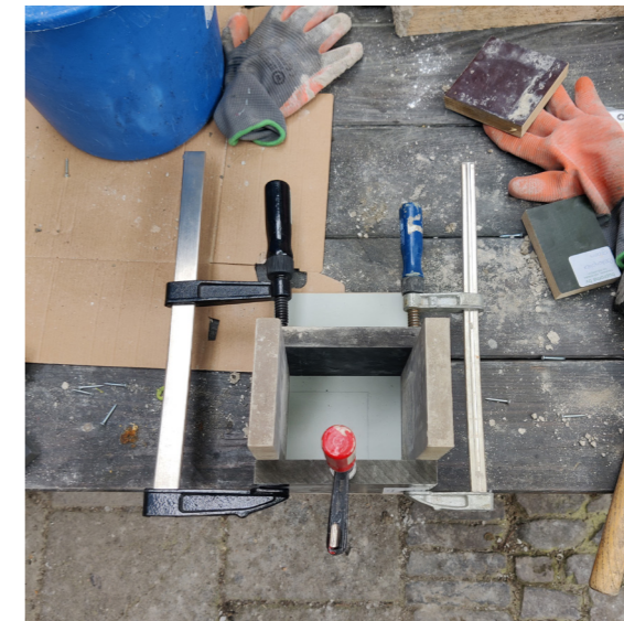
Step 6 / The formwork/mould is made from non stick wooden panels, held together by clamps. First I used screws, but to enable easy demoulding clamps work better, also not damaging the formwork.
