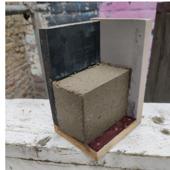
Step 11 / Remove the formwork The positives about a sample of this size is that you can also remove the formwork immediately, this allows it to harden faster and when making a lot of samples you could start with another one right after.
