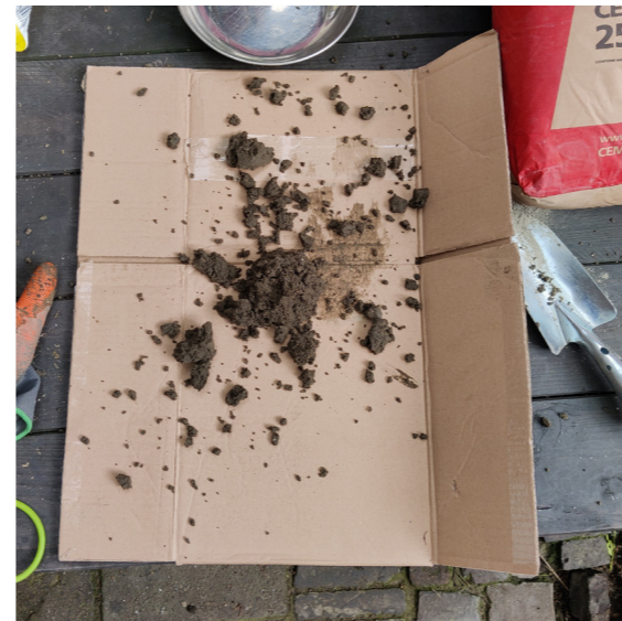
Step 5 / The ball should then be dropped from about a meter's height and break into a few larger and smaller pieces. If it doesn't break into pieces or the particles are the same size or too small, it is probably a sign that the water content isn't right. Too much water and the ball stay together when dropped, too little and it just result in sand on the floor.
