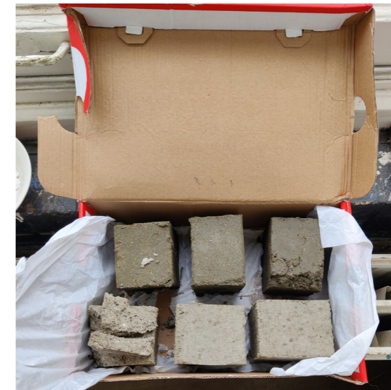
Step 12 / The next week or two is when the wall is at its most fragile stage. It will also change colour and by how much, depends on your mix, choice of cement and the dredging specie ratio.
