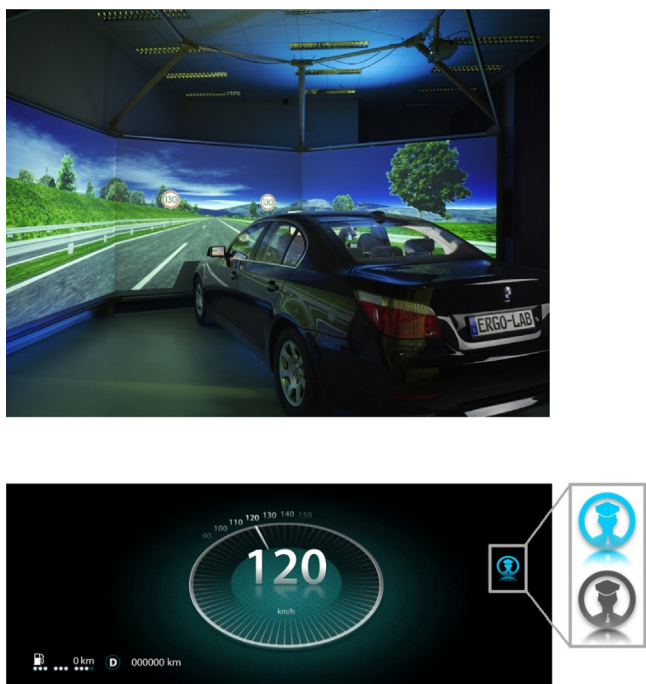
Fig. 1. Top: Driving simulator used in this study. Bottom: The visual display shown on the instrument cluster of the simulator. The center showed the speedometer, and on the right side an icon indicated the automation status (blue icon = active; grey icon = inactive). (For interpretation of the references to colour in this figure legend, the reader is referred to the web version of this article.)
