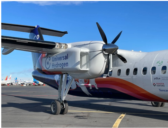
Figure 1.4: Prototype of fuel cell powered aeroengine. Cooling ram air ducts clearly visible. Credit: Universal Hydrogen.
