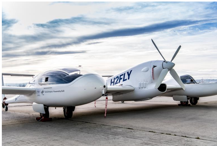
Figure 2.1: HY4 test airplane during testing in Stuttgart (Source: H2Fly) [33].
