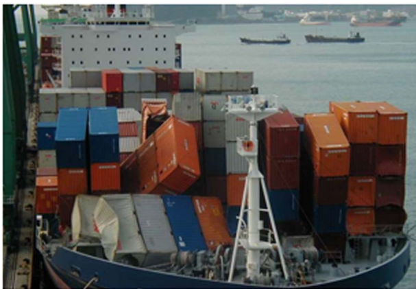
Fig. 3 Green water damage observed in the port of Busan, South Korea on “P&O Nedlloyd Barcelona” after a heavy storm on the North Pacific. Reproduced with permission from Ref. [21], courtesy: Shipspotting admin P. Melissen / hwnautic.
