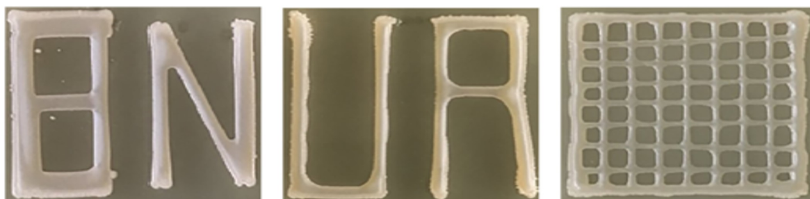
Figure 2.8: Geometries printed using direct ink writing and the ink formulation developed by Balasubramanian et al.[4].
