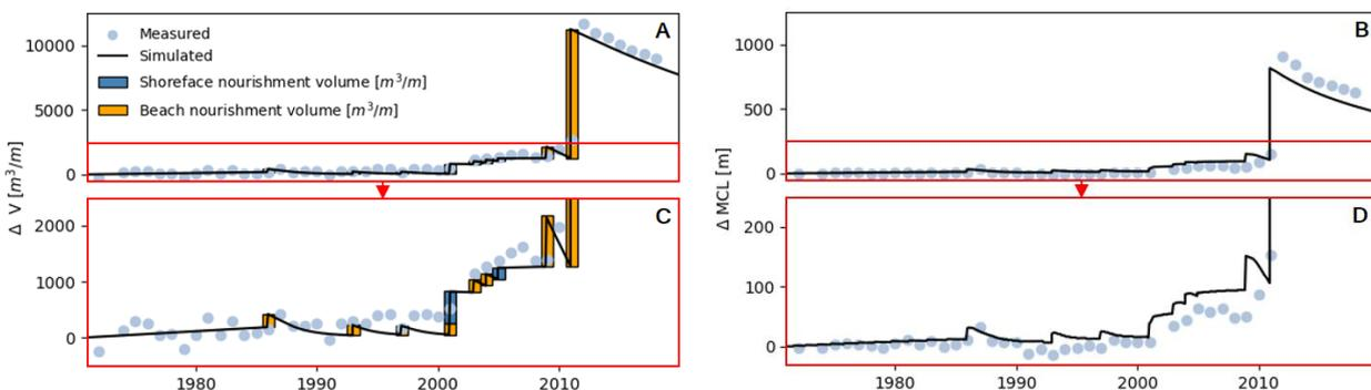
Figure 3 - Hindcast and measurements of active profile volume change  $\Delta V$  and momentary coastline change  $\Delta MCL$  at Monster (the Netherlands). Vertical close ups of panel A and B are displayed in panel C and D respectively.
