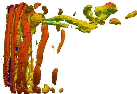
Figure 4.28: Iso-volume plot of the side view of the Goettingen 803 turbine in the AL-BEM simulation
