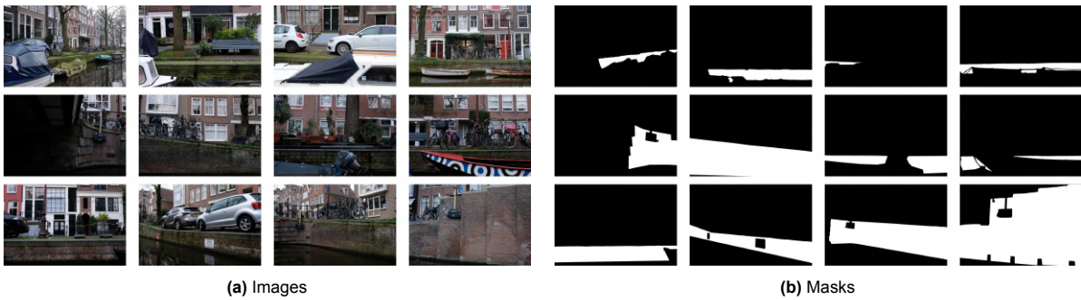
Figure 3.3: (a) A selection of images from our quay wall dataset, containing a total of 200 data pairs, (before augmentation processing) and (b) corresponding masks.
