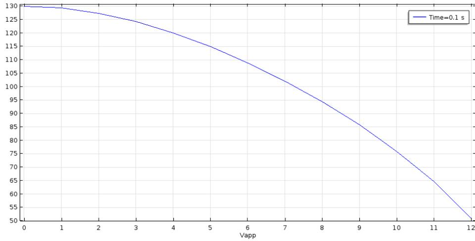
**Figure 3-4** Contact angle calculated by the TPF physics as a function of the applied voltage
