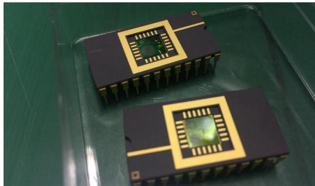
**Figure 5-3** Chips in the DIL24 package
