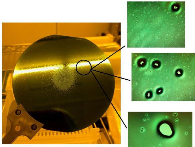
**Figure 4-14** Bubbles and holes on spray coated Photoresist results (1 layer)
