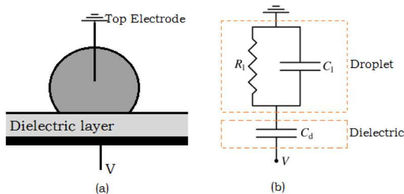
**Figure 2-5** (a) A droplet with separate electrodes EWOD configuration (b) equivalent simplified circuit diagram.
