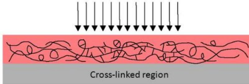
**Figure 4-10** Scheme of crosslinking [22]
