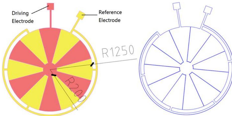
**Figure 4-2** Mask for Electrode Pattern Version One
