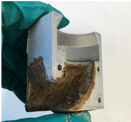
Fig. 12. The stiff material got stuck in the nozzle during the waiting period of the open time test, which is one of the reasons to restrict the printed amount.
