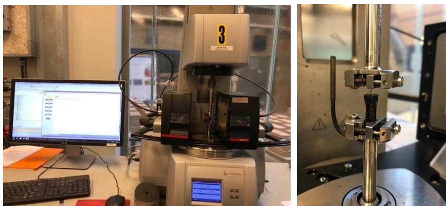
Figure 2.10. (Left) Anton Paar MCR machine + Data acquisition system and (right) specimen mounted to the clamping system
