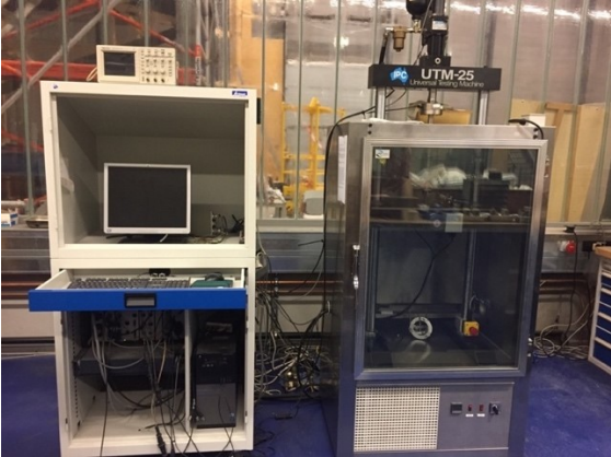
Figure 3.4. UTM25 + Data Acquisition System
