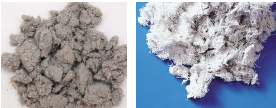
Figure 1.3. Cellulose (left) and mineral (right) fibres
