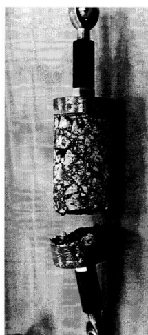
Figure 3.1. A direct tension specimen with failure occurring nearby the end cap [37]
