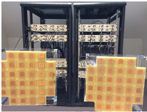
(a) The two distributable 32-antenna arrays in our testbed.
