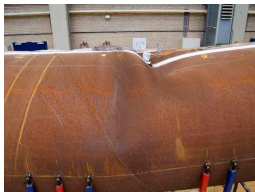
(b) Local buckle in specimen T11 ( D/t=83 )
