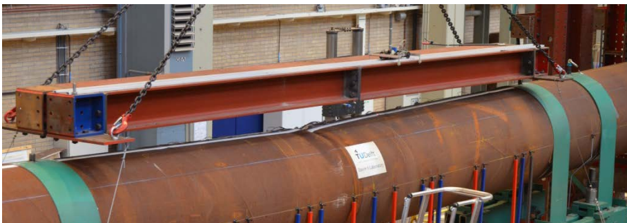
(b) Suspended rails for external laser equipped trolley
