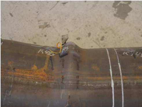
(c) Pressurized specimen T5 (right side of the fault)
