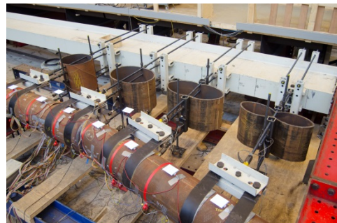
(b) Pipe-soil interaction by ring-springs (test 8)
