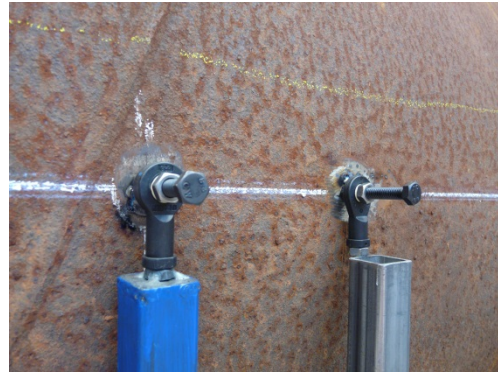
(b) Attachment of the measurement brackets to neutral line with a ball hinge
