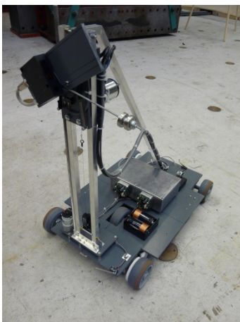
(a) Front of the trolley with rotating laser
