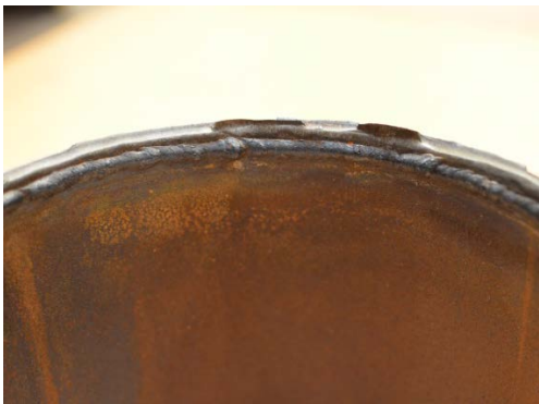
(c) Close-up of rupture surface near weld
