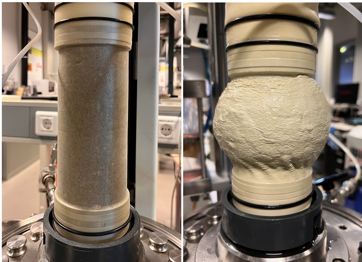
(a) Prepared sample before test.
