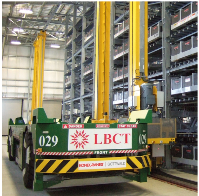
Fig. 1. Battery swapping stations are used to swap depleted batteries from AGVs [16]
