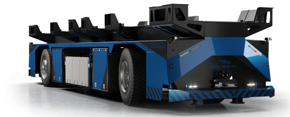
Figure 2.4: A conceptual AGV developed for Container Terminal Operations by Gaussin [29]
