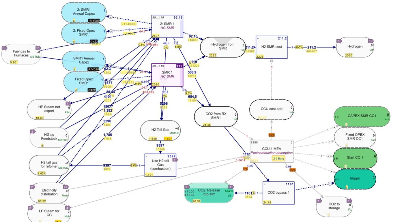
Fig. C3. Steam methane reforming + CC block in Linny-r.
