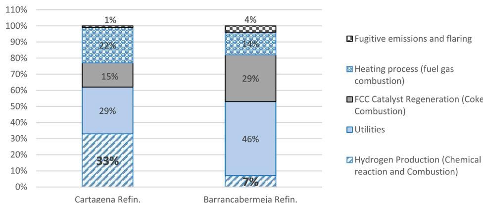
Fig. 1. Refinery CO<sub>2</sub> eq emissions allocation by origin. Source: (Ecopetrol, 2021).
