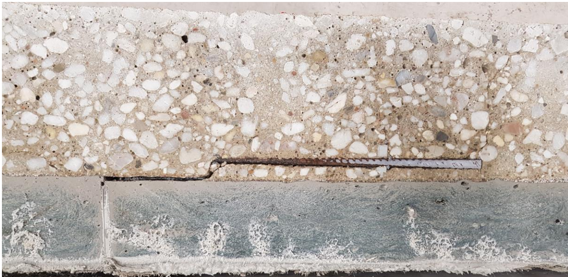
Figure 3-147: Crack propagation of the sample with epoxy and sand at the interface
