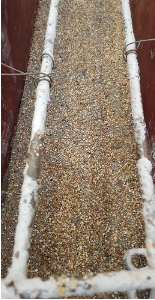
Figure 3-31: Interface with Epoxy and Sand
