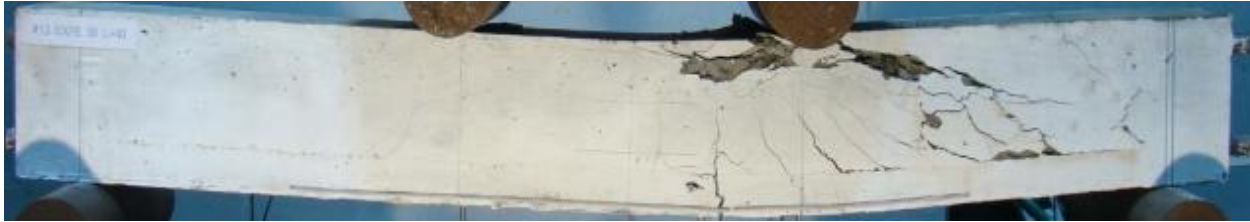
Figure 2-19: Failure of the strengthened samples with a 20mm SHCC layer (top) and 40mm SHCC layer (Hae Jun Yang et al., 2011)
