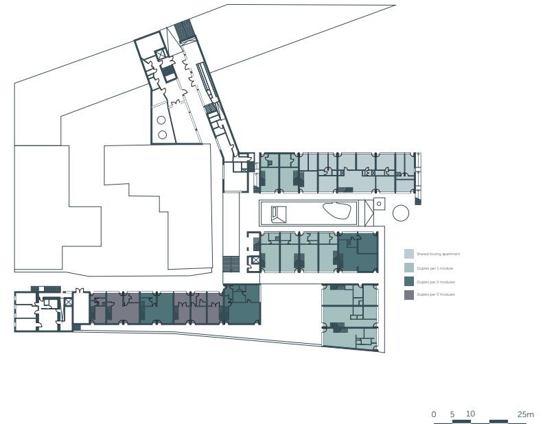
Analysis 12: Placement of units on ground floor (source: own illustration, adapted from https://issuu.com/nushratj/docs/sargfabrik_booklet )
