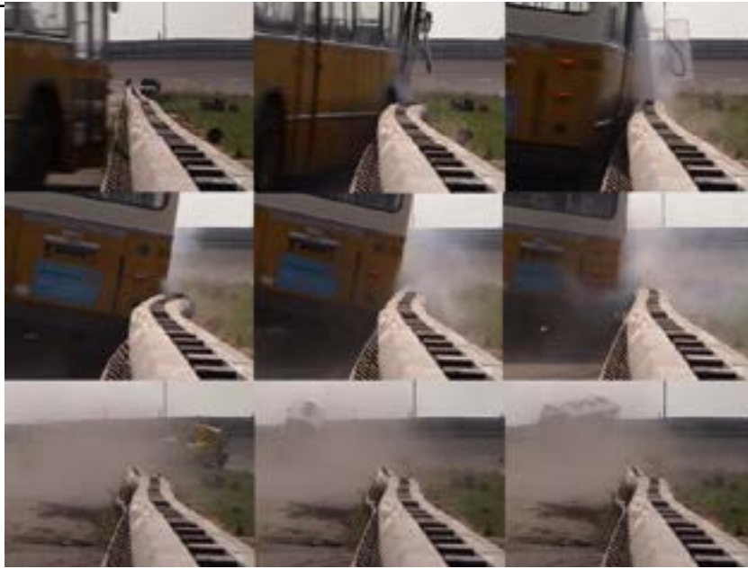
Figure 8. Back view from a full-scale test with a bus. No damage to the timber, except a need for straightening, saving repair time and costs.
