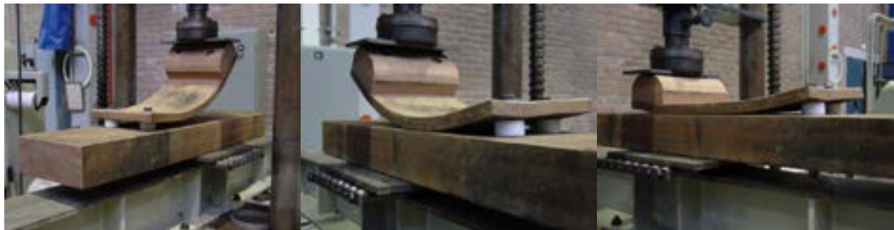
Figure 4. Three stages of bending of the steam bent element with car rail, connected to the pile with two bolts and white coloured spacers.
