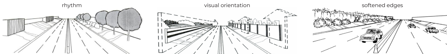
Figure 10.1: A selection of aesthetic principles in barrier design (Farnham et al., 1990)
