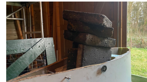
Figure L4: Prototype carrying 120 kg worth of tiles
