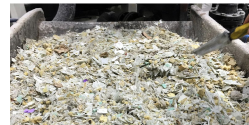
Figure 5.5: Shredded blades for cement production (Recharge, 2020)
