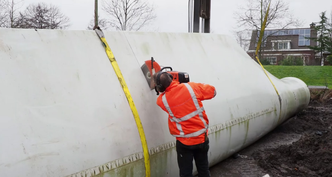
Figure 8.1: Segmenting a blade using straight cuts (GKB Groep, 2021)
