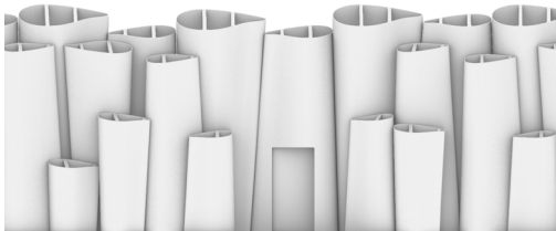
Figure 22.5: Traditional escape door integrated in Blade Barrier
