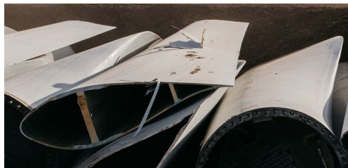
Figure 4.2: blade cross section (Bloomberg, 2020)
