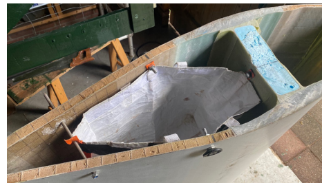
Figure L2: Connection of the bag to the segment
