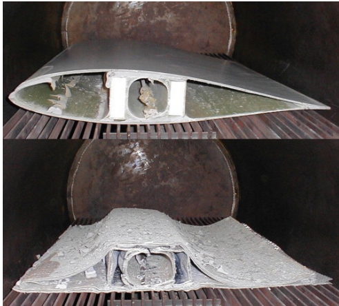
Figure 5.6: A blade segment treated in a pyrolysis reactor (Larsen, 2009)
