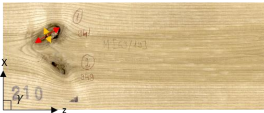
Figure 2: A real board with a knot. Red arrow is the maximum diameter and the yellow arrow is the minimum diameter of the knot
