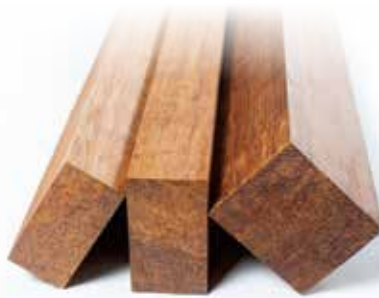
Figure 10. Strand woven bamboo beams are made by compressing rough bamboo fibres in moulds under very high pressure.
