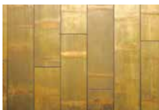
Figure 12. Flattened bamboo features the original bark of the bamboo stem as top layer.
