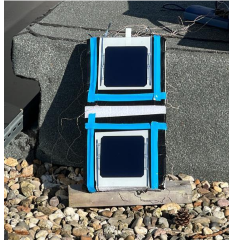
Figure 18- Setup configuration of prototypes with tape insulation on the sides
