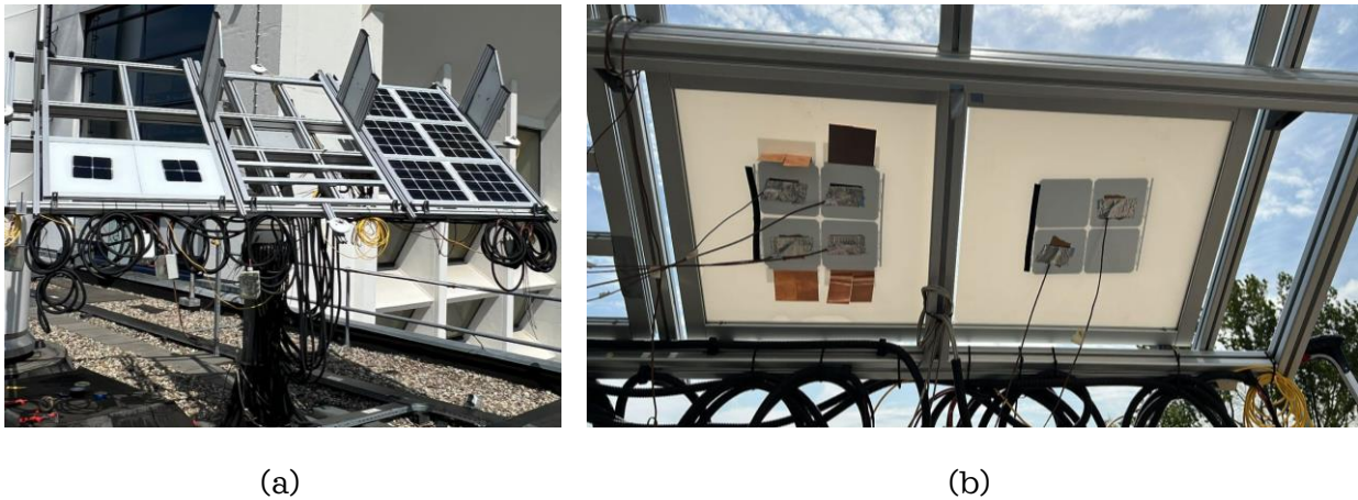
Figure 40- a) Setup for test procedure on May 8, 2022 b) Thermocouple connections for test on May 8, 2022
