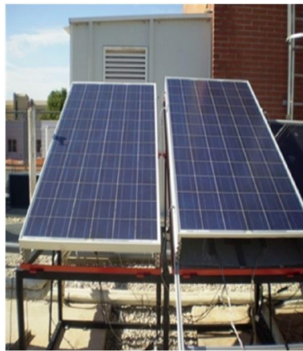
Figure 2 -Natural convection configuration of passive air stream (Mazón-Hernández, García-Cascales, Vera-García, Káiser, & Zamora, 2013)
