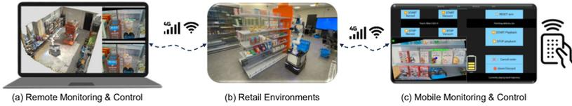
Figure 8.10: Overview of the remote monitoring and control system. a) Laptop-based remote interface for monitoring and control system; b) Visualization of the robot within the actual retail environment; c) Tablet interface for on-the-go monitoring and task programming.
