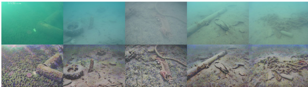
Fig. 4 The top row showcases the original images from different data collection sites of our dataset, while the bottom row displays the corresponding Fusion enhanced versions. A more uniform color distribution can be observed in the Fusion-enhanced images.
