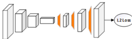
Figure 3.7: Pose estimation baseline model architecture [11]
