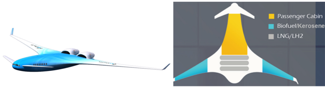
Figure 23. The multi-fuel blended-wing body investigated in the AHEAD project [37].
