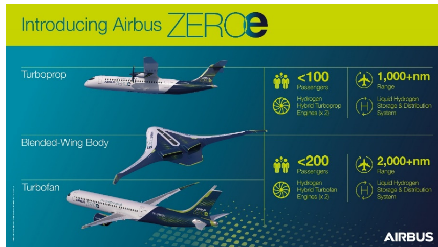
Figure 22. The three aircraft concepts from Airbus using LH 2 as an energy carrier to reduce the environmental footprint of aviation.
