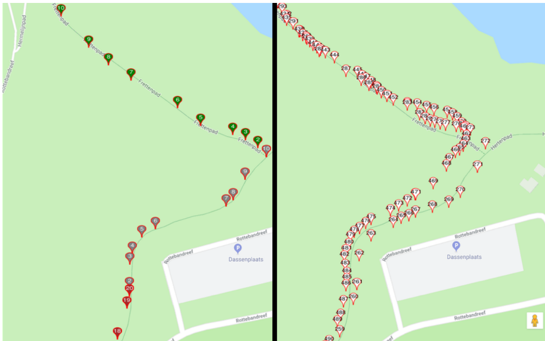
Figure 18: Correctly snapped waypoints: the right side contains GPS locations, the left side the matched points.
