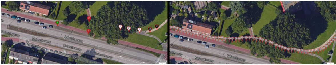
Figure 17: Badly snapped waypoints: the right side contains GPS locations, the left side the matched points.
