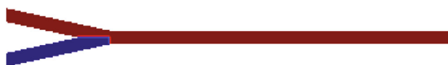
FIGURE 6 Flow initialization in all simulations. The red fluid is the aqueous phase and the blue fluid is the organic phase. [Colour figure can be viewed at wileyonlinelibrary.com ]
