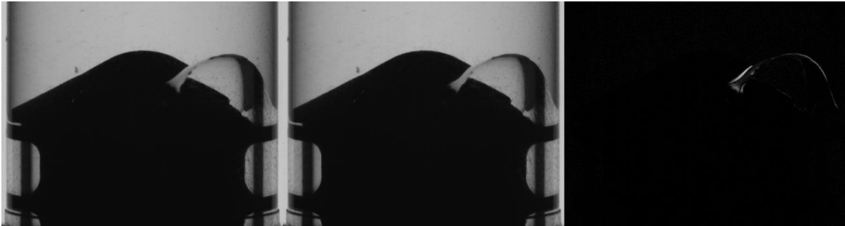
Figure 38 Left and Centre: Cropped section of a syringe with a bubble on the rubber stopper on two subsequent frames. Right: Absolute difference between the two frames.
