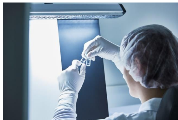
Figure 2 Manual inspection process with white and black backgrounds to detect different types of particles. Source: [38]
