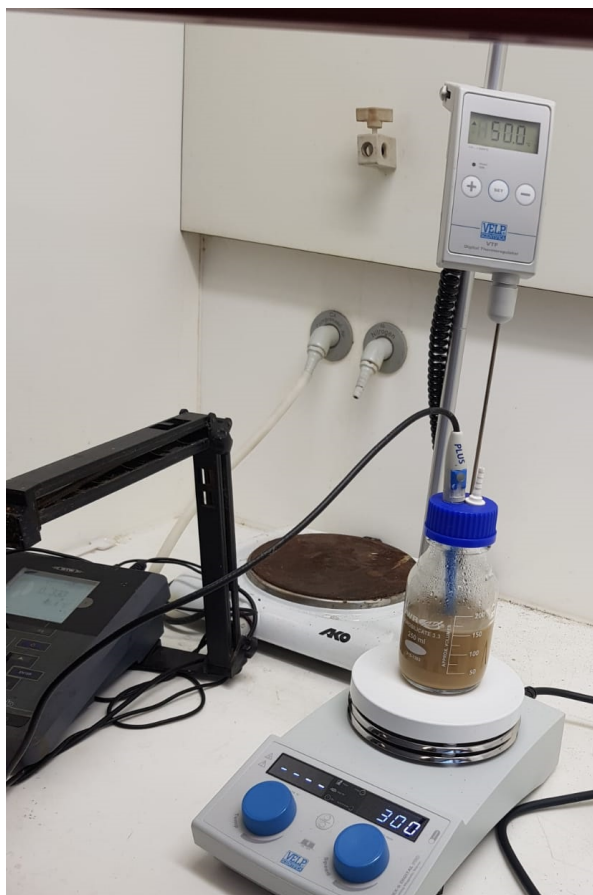
Figure 4.8: Setup for leaching experiments: 250mL borosilicate glass jar with holes drilled in caps for the temperature probe, pH meter and for sampling. Jar was placed on a hotplate/magnetic stirrer which was connected to the temperature probe.
