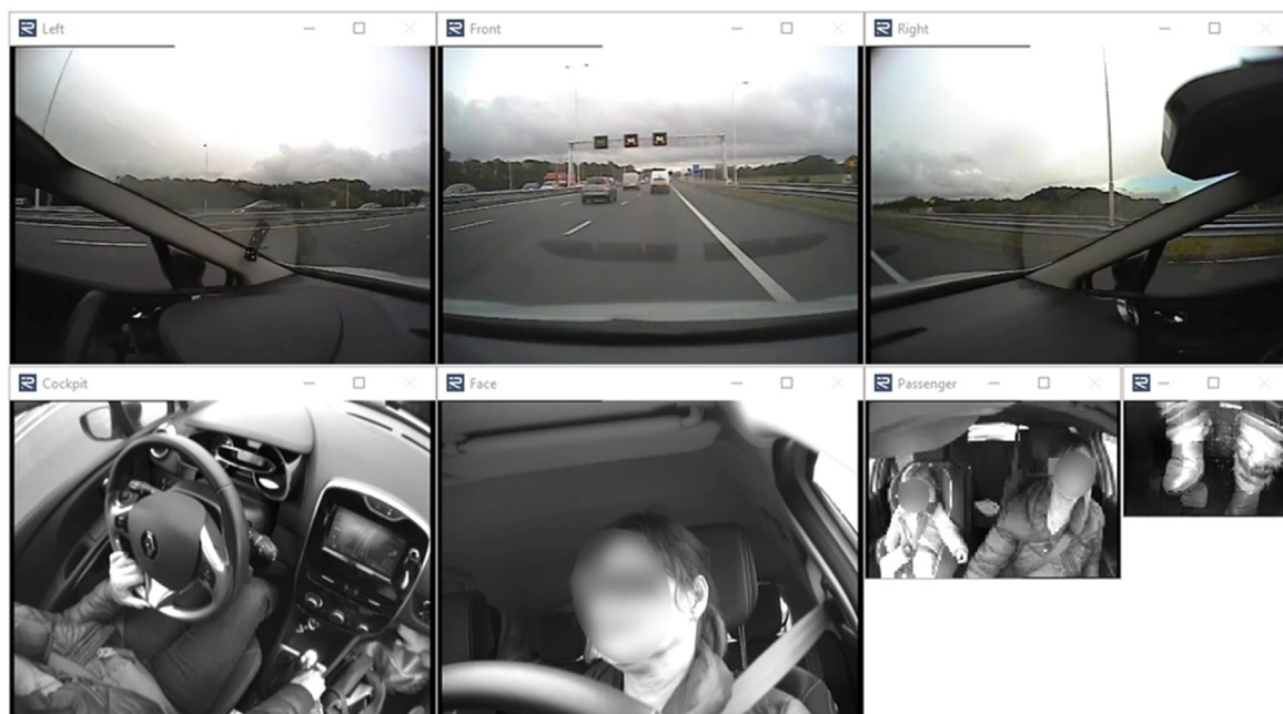
Fig. 1. Seven camera views of the UDRIVE database at the encounter of an active VSL: front left, front centre, front right, cockpit, driver face, cabin, and feet. Faces have been covered to respect the privacy of the participating driver and passengers. This figure was originally presented in Varotto et al., (2021) .
