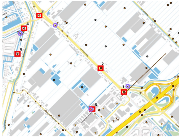
Figure 6.17: Boreholes(Red) and Cone Penetration Test Locations(Purple) in Nieuwerkerk aan den IJssel
