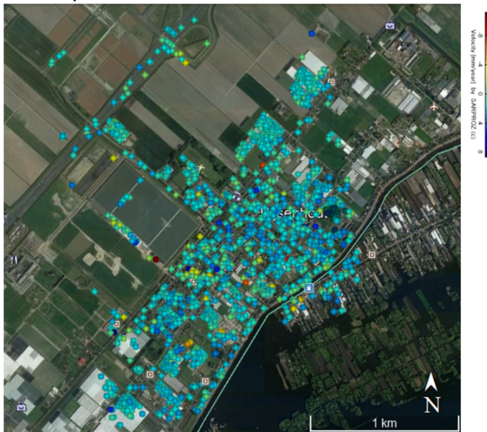
Figure 6.9: Persistent scatterers - InSAR Analysis in the area of a greenhouse in Schiphol
