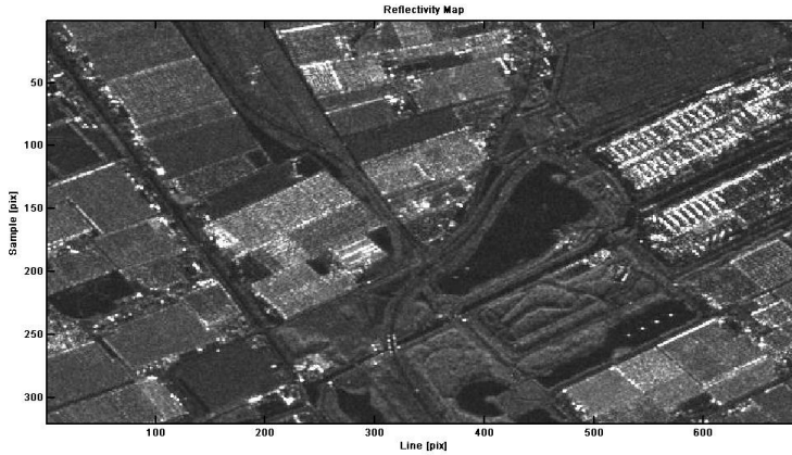
(a) Reflectivity map visualised by the computation of the average of the amplitudes of all images in the data-stack, in this case of 28 Radarsat-2 images covering a scene with greenhouse 'Westland A'
