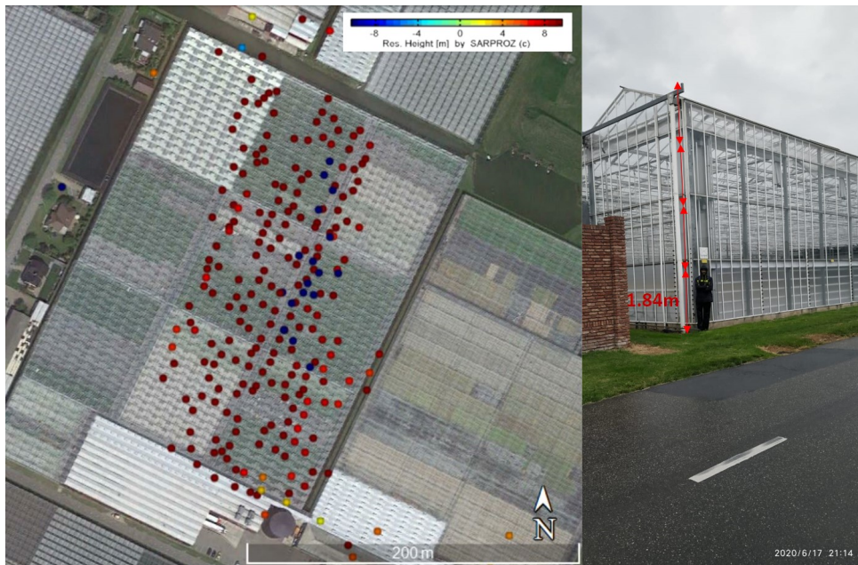
Figure 6.40: Residual heights of the persistent scatterers for greenhouse 10 (L), investigation of greenhouse's height from field visit (R)
