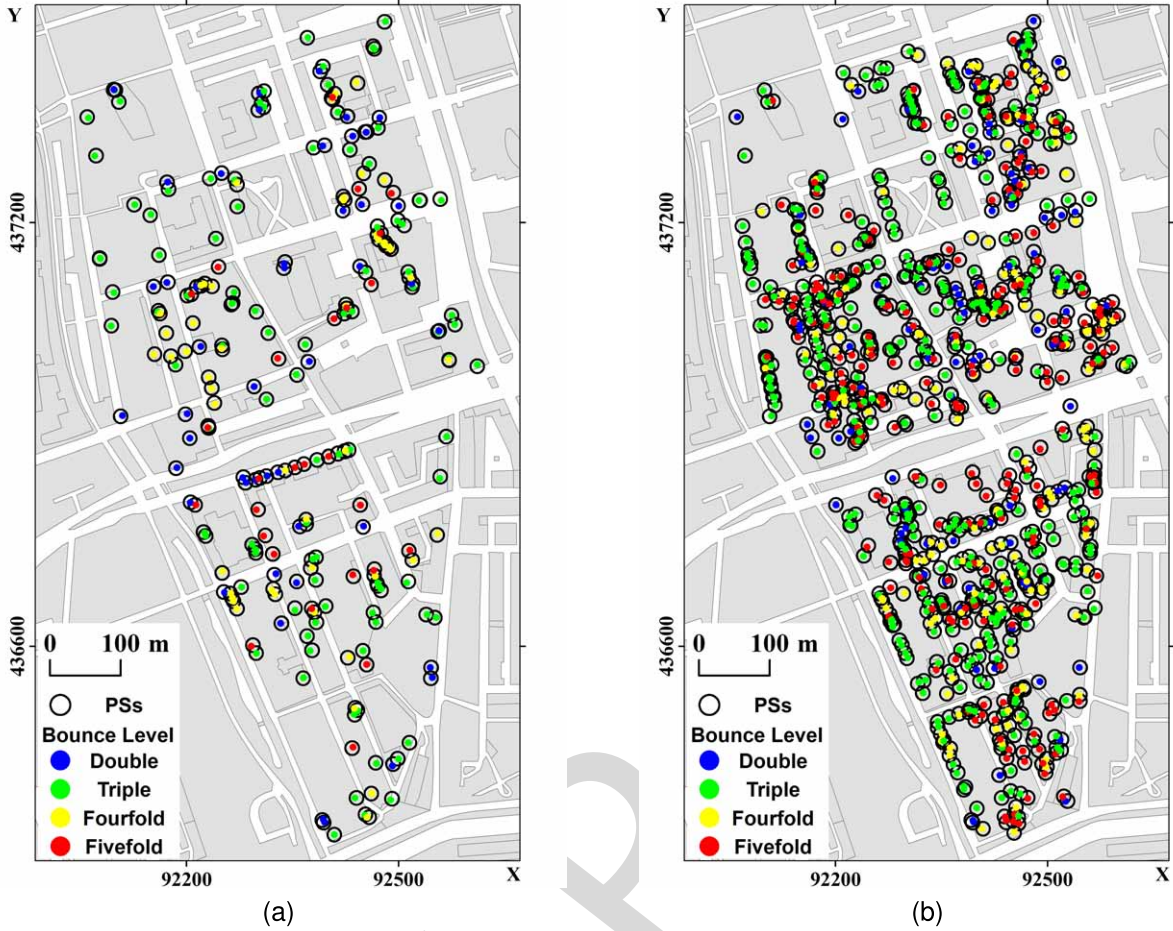
Fig. 11. Correspondence between SPSs, shown as solid circles color-coded by bounce level, and matched PSs, shown as empty circles. (a) Left and (b) right correspond to simulations using the LOD1 and LOD2 models, respectively.
