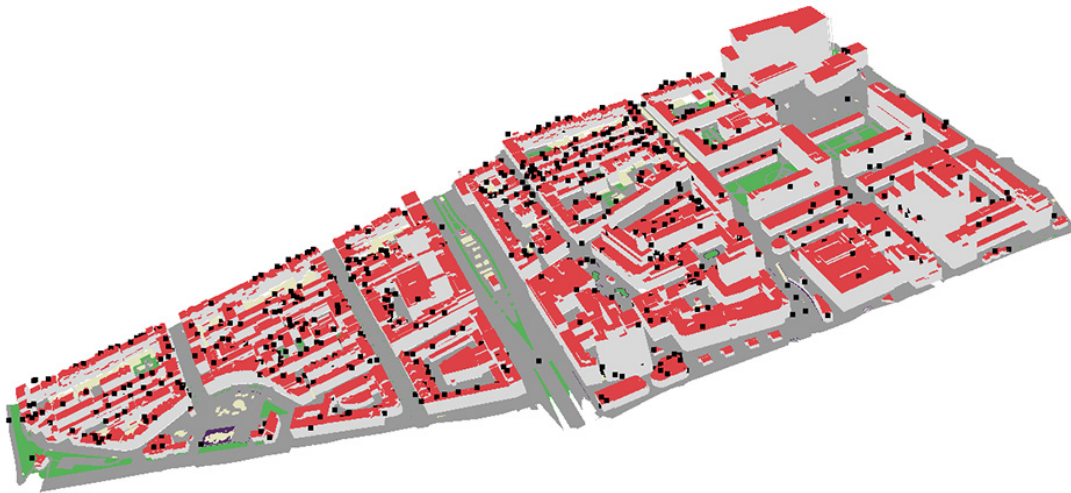
Fig. 15. Rendering of matched scatterers overlaid on the LOD2 city model.
