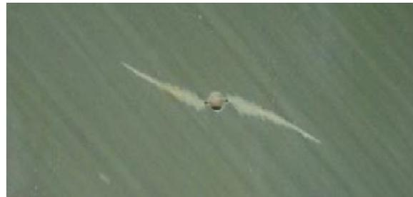
Figure 5.16: Delamination around the crack of a GLARE 2A specimen under  $S_{max} = 140$  MPa and  $R = 0.05$  at  $OAA = 45^\circ$  [34]
