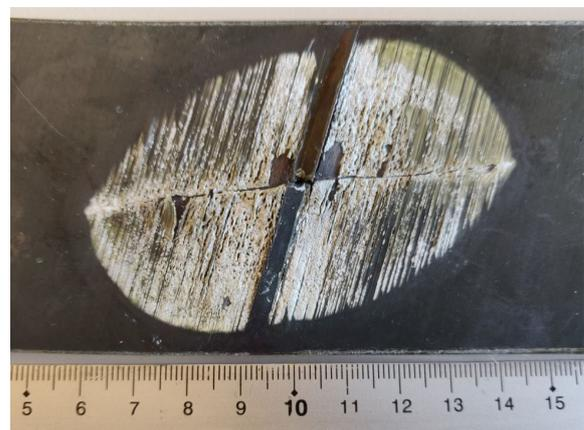
Figure 4.19: Test 5 delamination contour after 160 kcycles (front side after etching)
