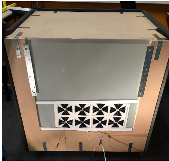
Figure 71 PV + PDLC system in OFF State
