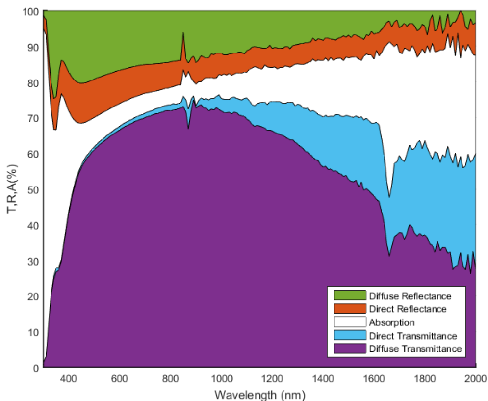
Figure 24 Transmission, Absorption and Reflectance of non-adhesive PDLC.
