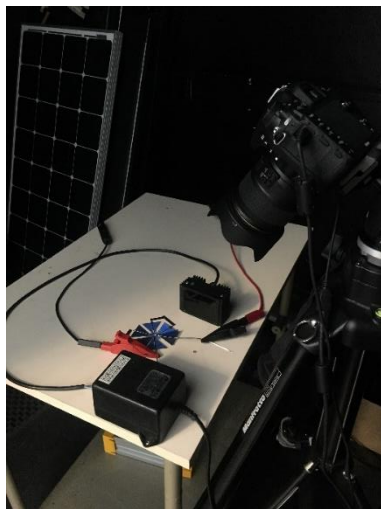
Figure 15 Camera and Mini module set-up for electroluminescence
