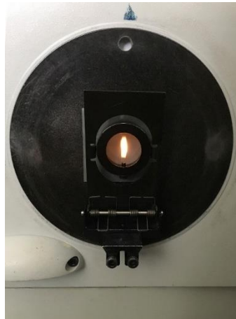
Figure 10 Reflectance set-up of the PDLC sample in the LAMBDA 950
