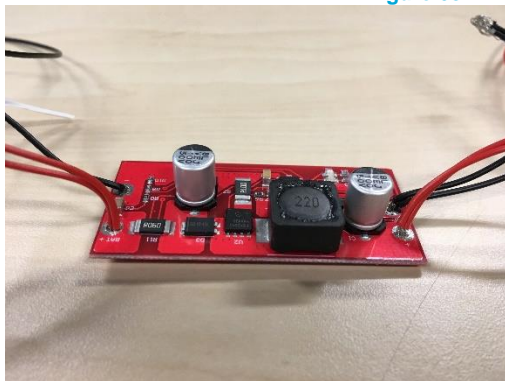
Figure 69 Charge Controller – MPPT for the system
