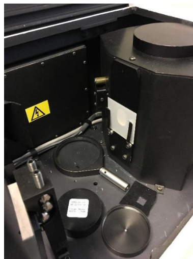
Figure 9 Transmittance set-up of the PDLC sample in the LAMBDA 950
