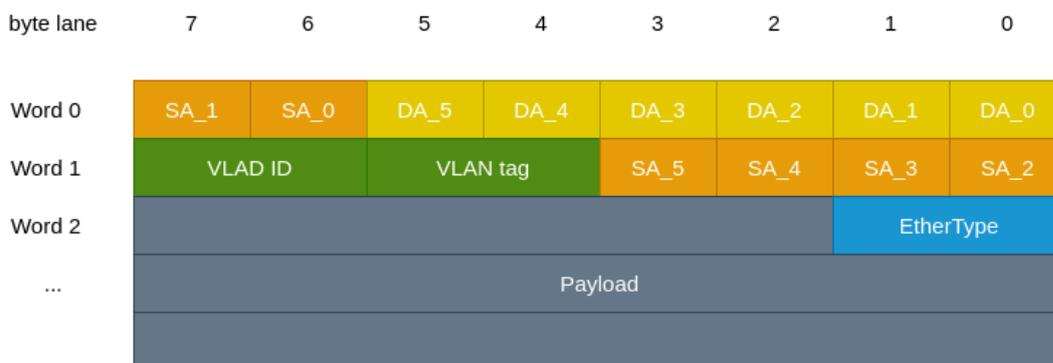
Figure 4.17: Typical structure of an Ethernet packet
