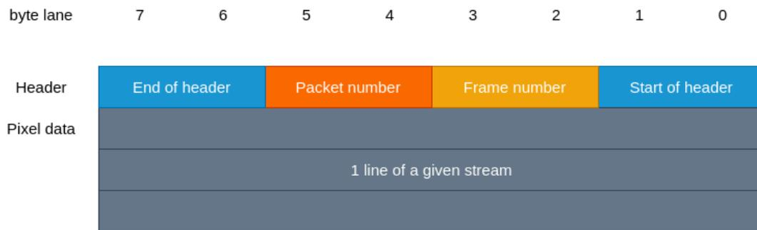
Figure 4.18: Typical structure of the payload
