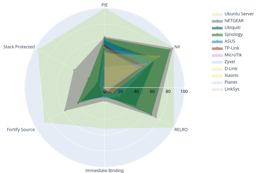
Figure 5.6: Exploit mitigation techniques IoT/embedded dominant Vendors versus Ubuntu Server 6 .
