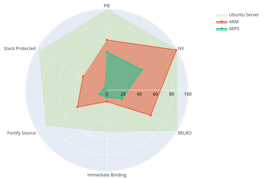
Figure 5.7: Exploit mitigation techniques ARM vs MIPS vs Ubuntu Server 6 IoT/embedded .
