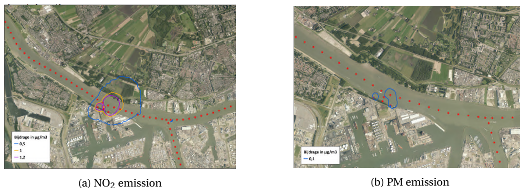
Figure 3.6: An example of a berth facility and its associated emission contours (Niemendal and Bouman, 2014)
