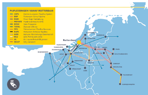
(a) Pipelines from PoR
