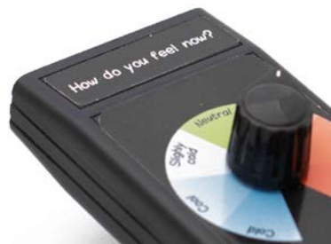
Figure 3.5: Comfort Dial used to capture comfort perception of the residential tenants
