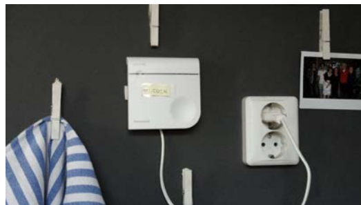
Figure 3.1: Temperature, Relative Humidity and CO 2 sensor box
