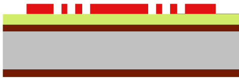
5. IDT patterning with laserwriter.
