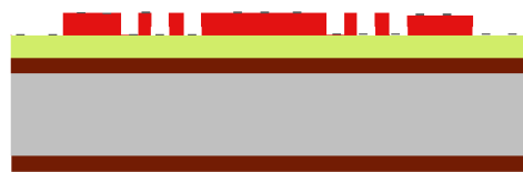
6. 10 nm Cr deposition (evaporation).
