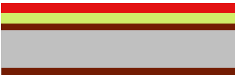
4. Coating with photo-resist.
