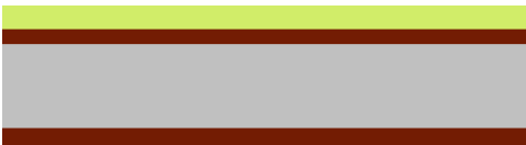
3. Deposition of 1 μm AlN on the front (Trikon Sigma 204).
