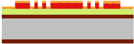
7. 90 nm Au deposition (evaporation).
