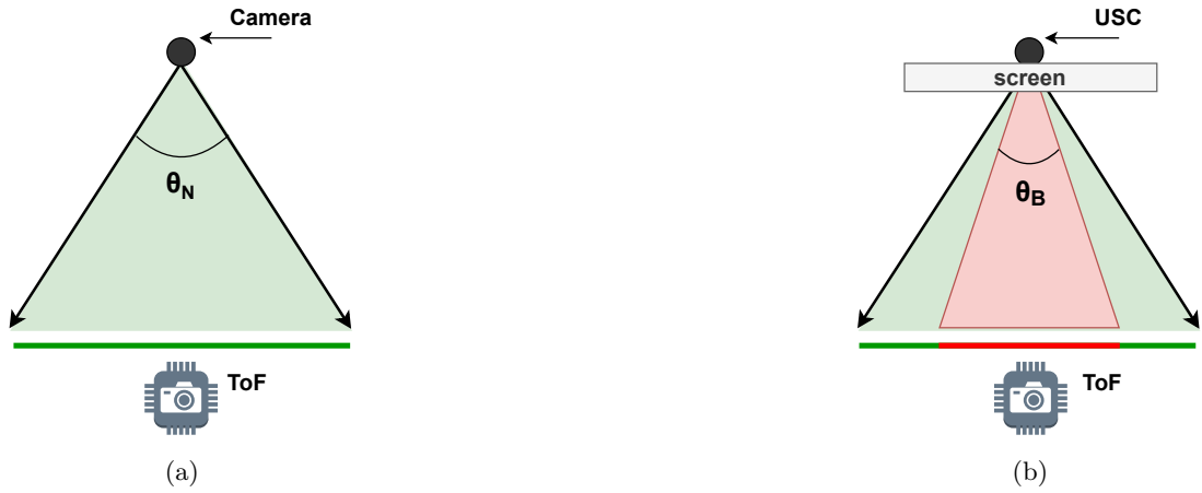
Figure 3.5: Effect of reflections from screen on the detectable FoV of the USC compared to situation with normal camera.
