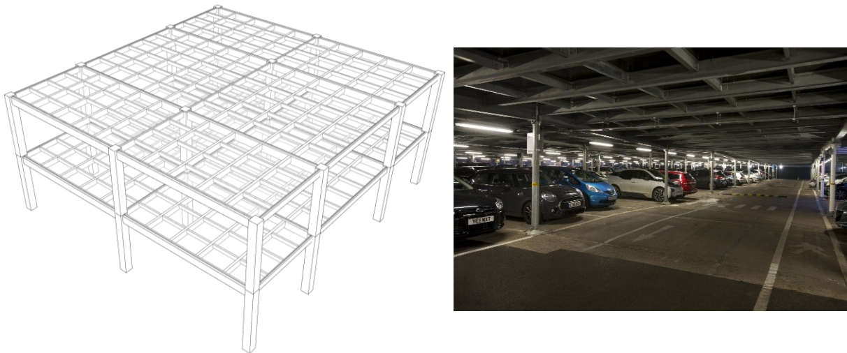
Figure 30. Girders across parking bays with primary and secondary joists supporting floor elements framing system (Osborne, 2019).
