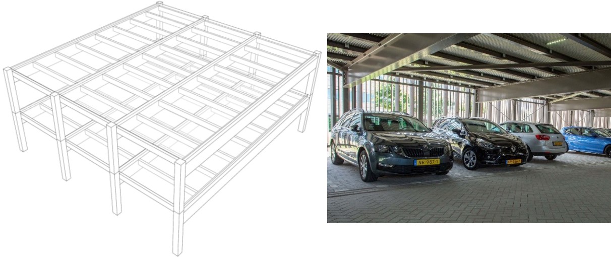
Figure 29. Bin wide girders with perpendicular joists supporting floor elements framing system (Park4all, 2019b)
