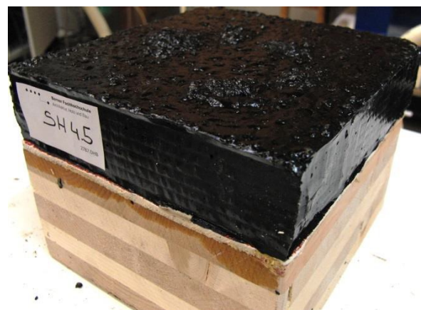
Figure 49. Test specimen of system with shear connection experiencing blistering (Scharmacher, Müller, & Brunner, 2014)
