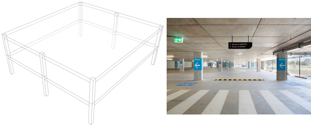
Figure 25. Two-way carrying slab framing system (AMC, 2021).
