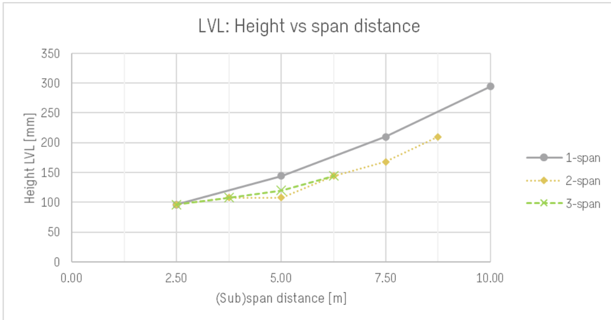
Figure 110. Comparison between single- and multi-span LVL systems for height vs span distance
