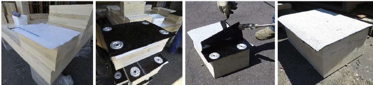
Figure 50. Test specimen of system without shear connection (Haynes et al., 2019)
