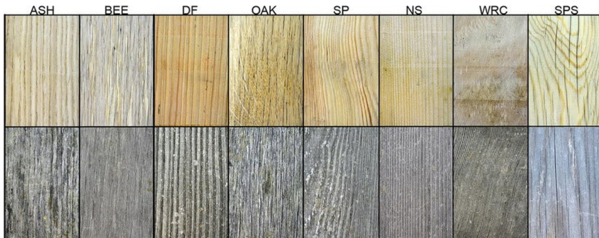
Figure 45. Weathering effects on timber specimens (Niklewski, Brischke, Frühwald Hansson, & Meyer-Veltrup, 2018)
