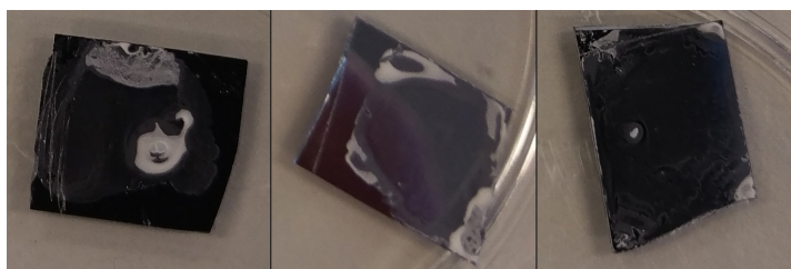
Figure A.1: Samples which have been plasma cleaned and spincoated with 100 \mu\text{l} of the aqueous polystyrene solutions. From left to right; 500 rpm, 1000 rpm and 2000 rpm spincoated for 60 seconds. All samples are around 1 \text{cm}^2 .
