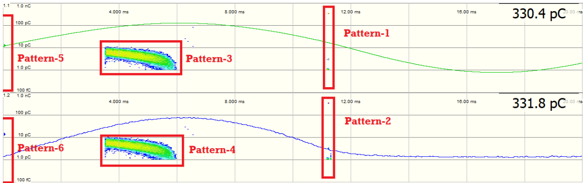
Figure 4.19: Histogram of the noise in negative half-cycle voltage test with Omicron 1&2
