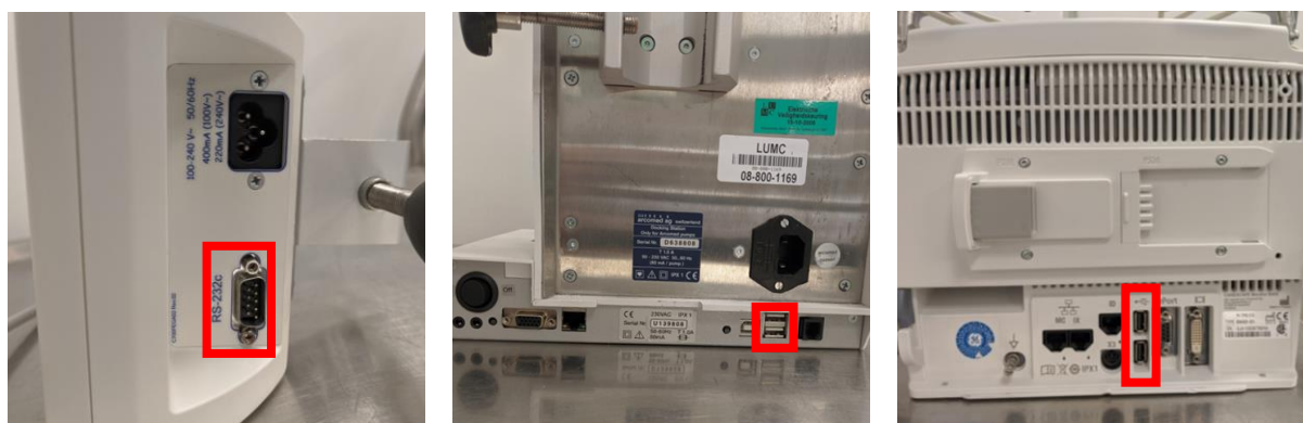
Figure B-1 Connection ports on TOF-Cuff (1a), Arcomed docking station (1b) and GE NMT monitor (1c)
