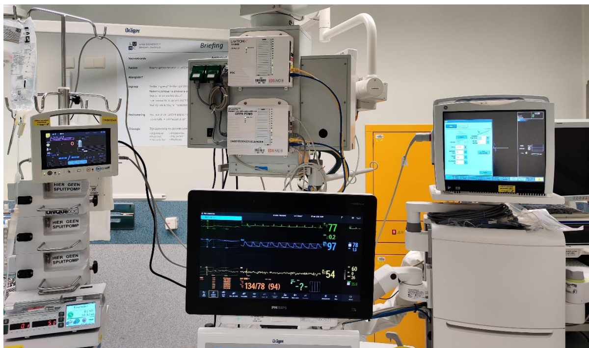
Figure 2-1 Experimental setup in the operating room, the Arcomed docking station with an inserted syringe pump is positioned on the lower left. On top of it, a TOF-Cuff is mounted to the pole. In the top middle, two Lantronix devices are placed, and on the right, a GE NMT monitor is positioned on top of a ventilator machine.
