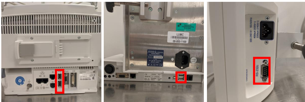
Figure 2-2: RS-232 ports on the GE NMT monitor (left), the Arcomed docking station (middle) and the TOF-Cuff (right).
