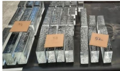
1. Bricks are categorized in height using a digital caliper.
