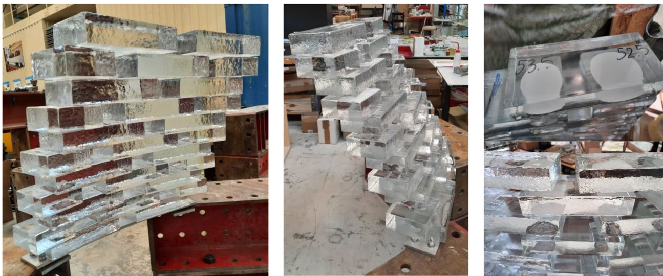
Fig. 18 Prototype constructed at the TU Delft Glasslab, showing the natural tilt of the bricks due to the larger cantilevering width in the initial design (left and center). The application of the DOWSIL
