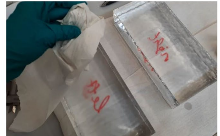
6. Bricks are removed and cleaned using isopropanol
