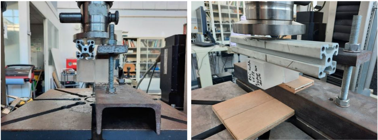
Fig. 10 Experimental set-up of the shear tests
